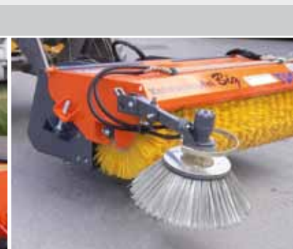
fully adjustable hydraulic side brush (50% PP / 50% wire)
